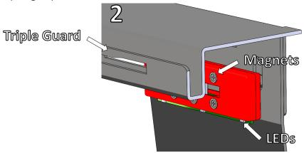
3. Attach the CV LED to the back of the triple guard with the magnets. Ensure that the L shaped locating feature is in the back hole of the triple guard and slid all the way to the left (**Image 3**).
