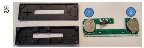
4. Place the PCB back in the case and secure the 4 screws. (Image 3).
