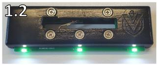
2. Place the CV LED behind the triple guard with the LED's pointing downwards and the magnets are facing the back of the triple guard (**Image 2**).
